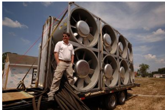
Figure 1.5a- Hurricane Simulator at UF [B7]
