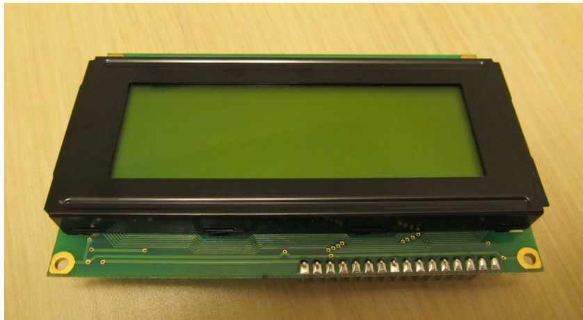
Figure 4.7.2a- This is the 4x20 character LCD that we are planning on using in the final project. As shown, it is a very simple display.
